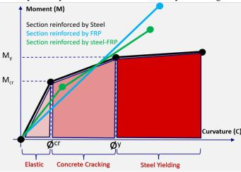
Figure 2. Schematic MC relation of hybrid-reinforced RC sections
