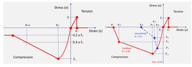
Figure 3. Different Concrete models implemented in this study
