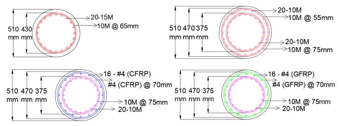
Figure 6. Cross section and reinforcement layout of the scaled models; (a) Steel (Control), (b) two layers of spirals (both Steel), (c) two layers of spirals (CFRP and Steel) and (d) two layers of Confinement (GFRP and Steel)
