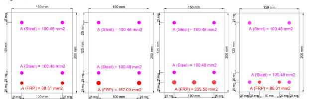
Figure 4. Cross section and reinforcement details
