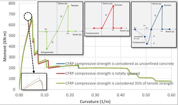
Figure 10. MC (Different approaches to model the compressive behavior of CFRP rebars)
