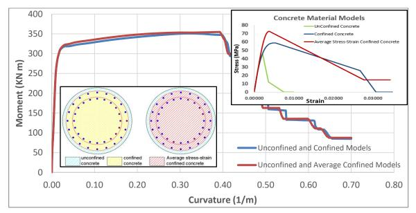
Figure 11. MC (Confined and unconfined concrete vs the average uniform confinement method)
