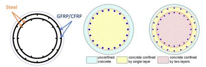
Figure 1. schematic cross-section, showing different confinement levels
