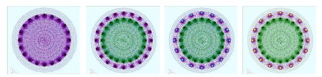
Figure 7. Mesh is tuned to precise element size near rebars while courser mesh is applied in other section parts
