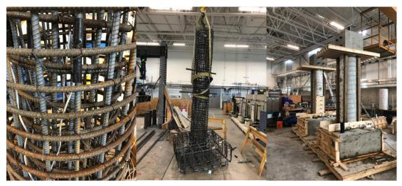
Figure 12. One and two layers of spirals specimens prepared for testing at ALAMS
