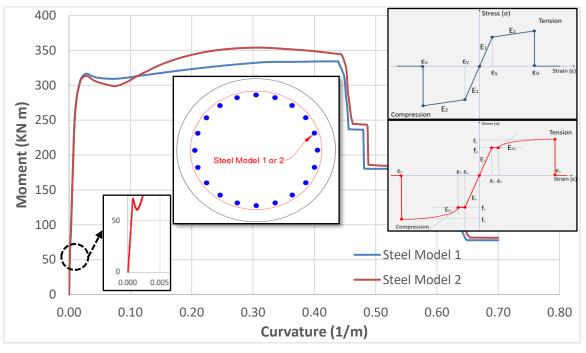
Figure 8. MC (bi-linear steel model vs nonlinear strain hardening steel model)
